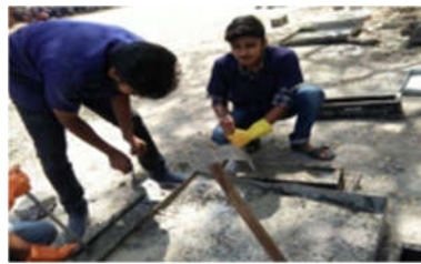
Figure 4.2 Compaction the prism mould
