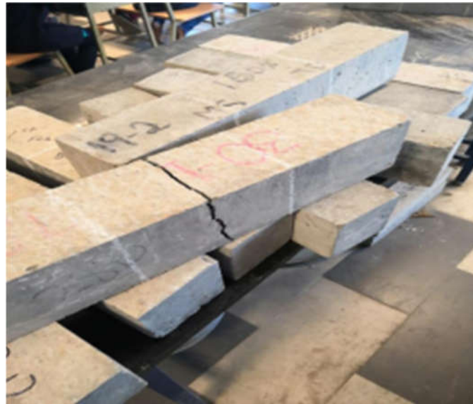
Figure 4.8 Tested concrete beam
