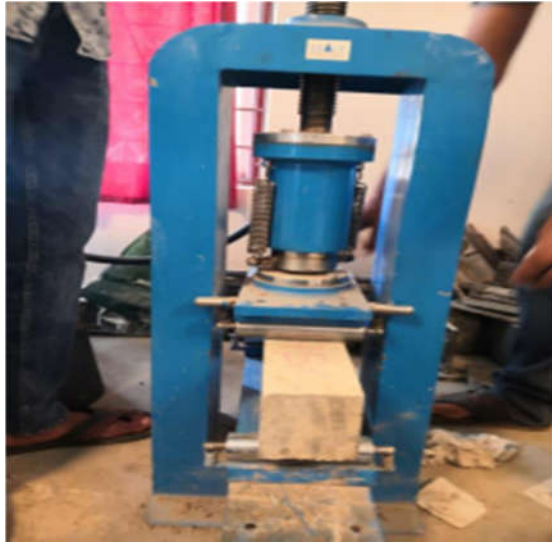
Figure 4.5 Flexural test on concrete beam
