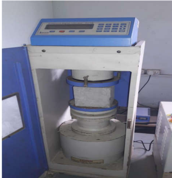
Figure 4.1 Compressive Strength test of cubes
