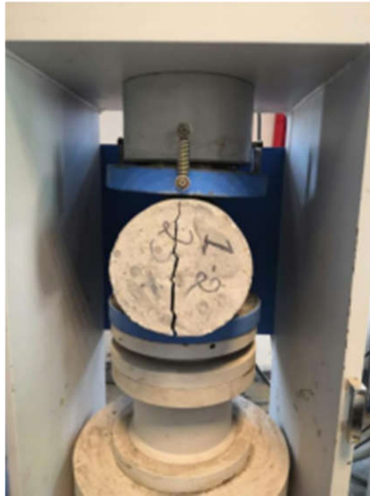
Figure 4.3 Split tensile test on concrete cylinder
