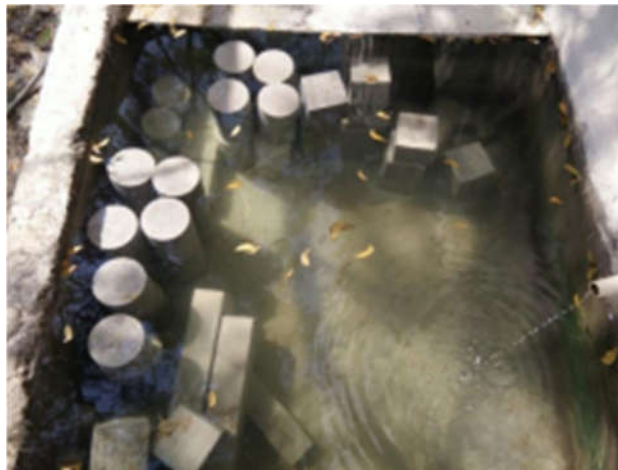
Figure 3.3 Curing the test Specimens
