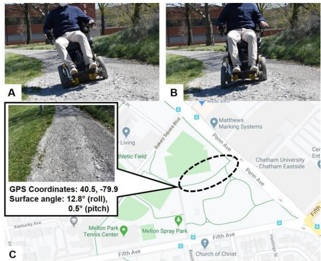
Figure 5. MEBot navigating over uneven terrains using passive suspension similar to EPWs (A) compared to MEBot using its self-leveling seat application for tip prevention (B). The MEBot's sensor package sends the location and surface angle to the eNav-Server (C).
