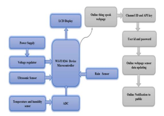
Fig no 4.1: block diagram for proposed system
