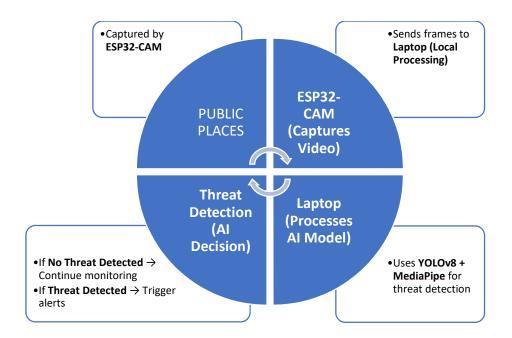
Fig 1: Basic Block Diagram.
