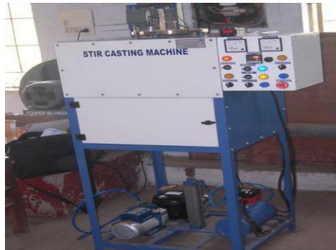
Fig 1:Stir casting setup
