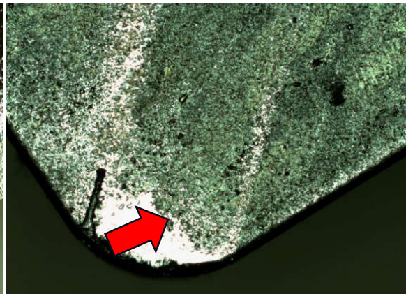
Fig 2. Rake Wear in Plane Cutting Tool Insert
