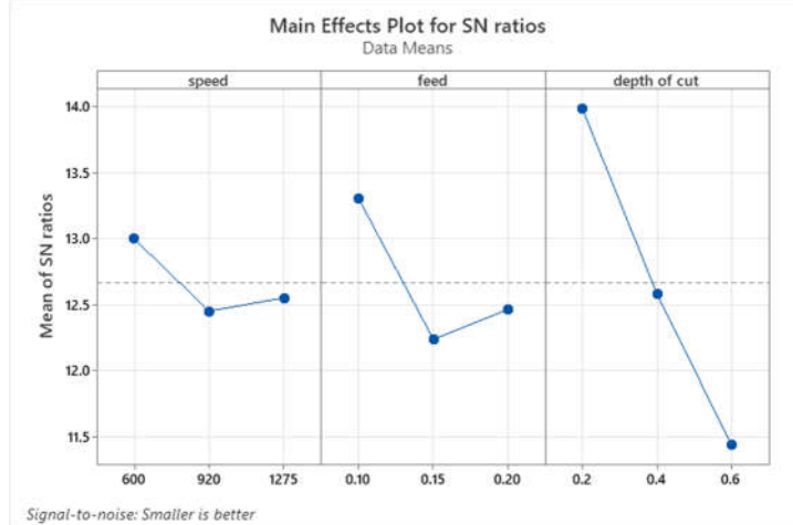
Fig 5. Effect of Cutting Speed, Feed Rate, and Depth of Cut on Tool Rake Wear under MQL for Plane Cutting Tool Insert
