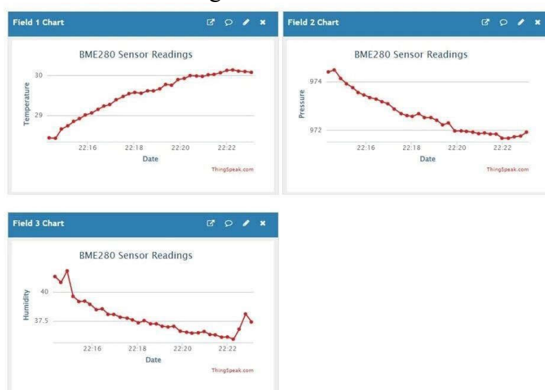
Fig 4 : IoT-Based Environmental Monitoring Dashboard in ThingSpeak
