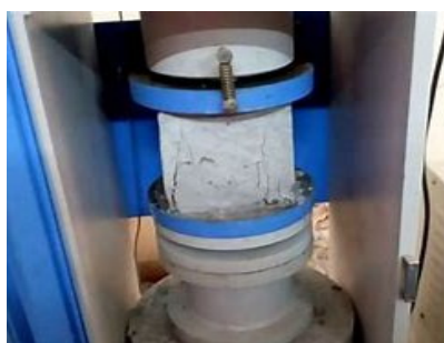
Fig. 4.1. Compressive strength testing machine
