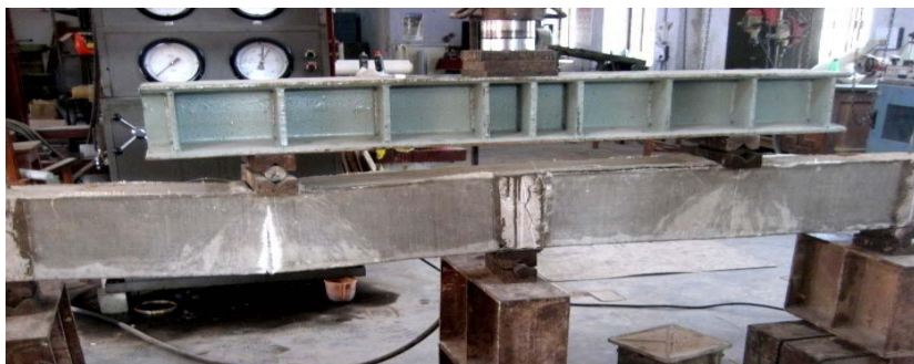
Figure 3.39 Failure of the beam by tensile rupture
