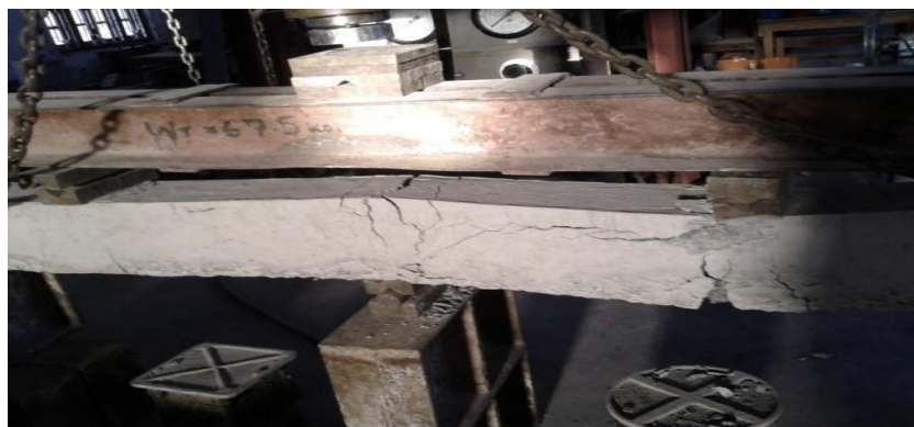
Figure 3.13 Control Beam, C.B2 after failure
