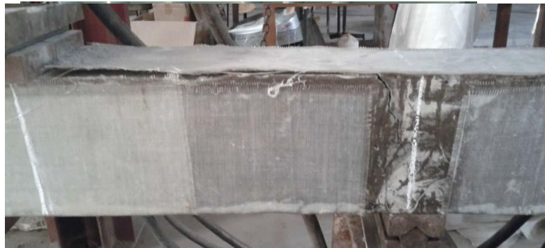
Figure 3.22 Crack pattern after initial loading
