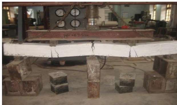
Figure 3.12 Flexural failure of C.B1
