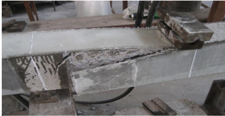
Figure 3.42 Shear crack in the left span
