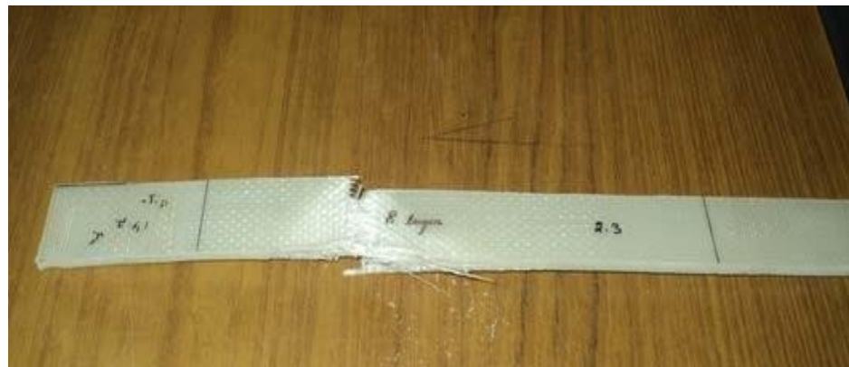
Figure 3.10 Specimen failure after the tensile test
