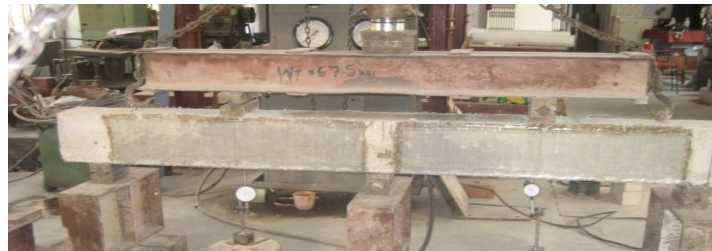
Figure 3.20 Debonding failure of FRP
