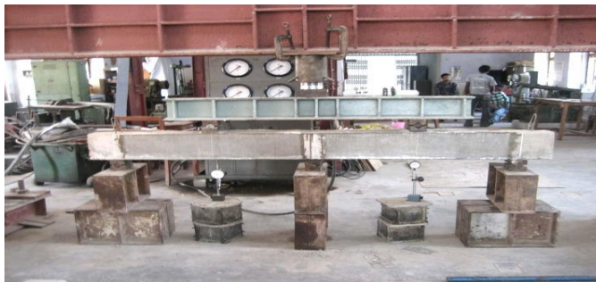
Figure 3.38 Experimental set up and strengthening pattern of TB2
