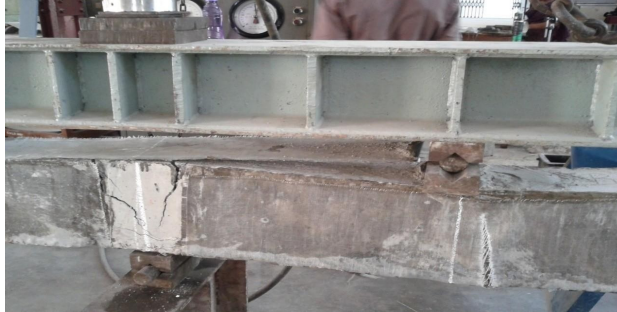
Figure 3.17 Tensile rupture of FRP at mid-section of right span at lower value
