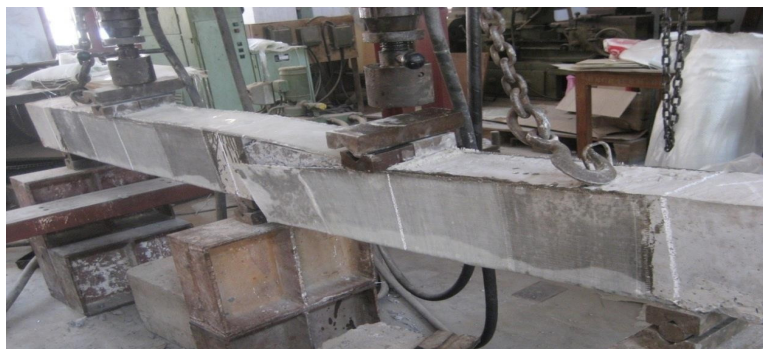
Figure 3.41 Failure of beam TB3
