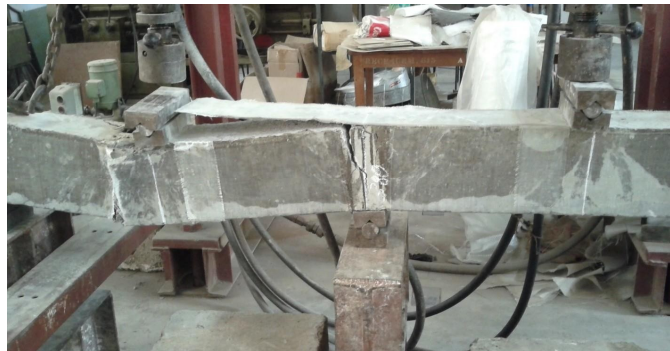
Figure 3.23 Failure of the beam by tensile rupture
