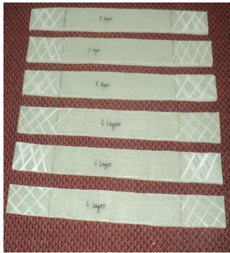
Figure 3.8 Specimens ready for tensile testing
