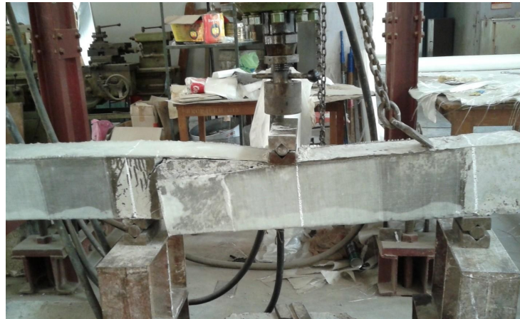
Figure 3.42 Shear crack in the left span
