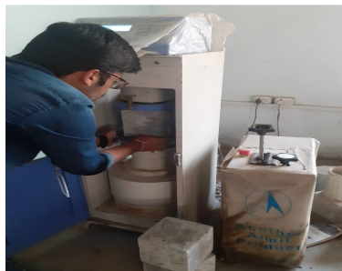
Fig 4.2: Performing Compression test for 10% replacement concrete cube
