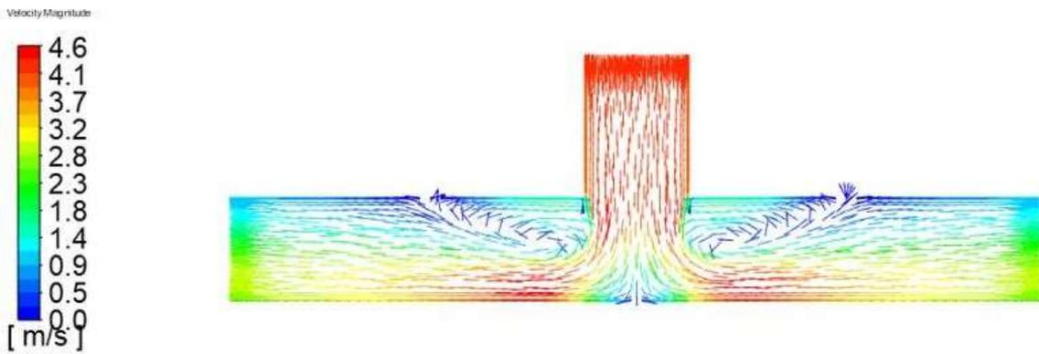
**Fig. Flow velocity of fluid in the manifold**
