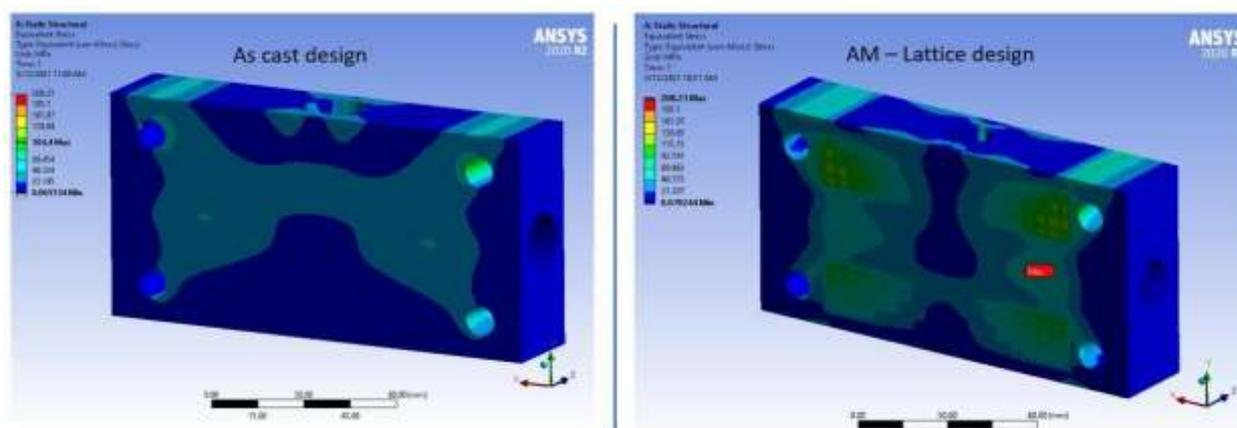
**Fig. Equivalent max. stress under pressure load**
