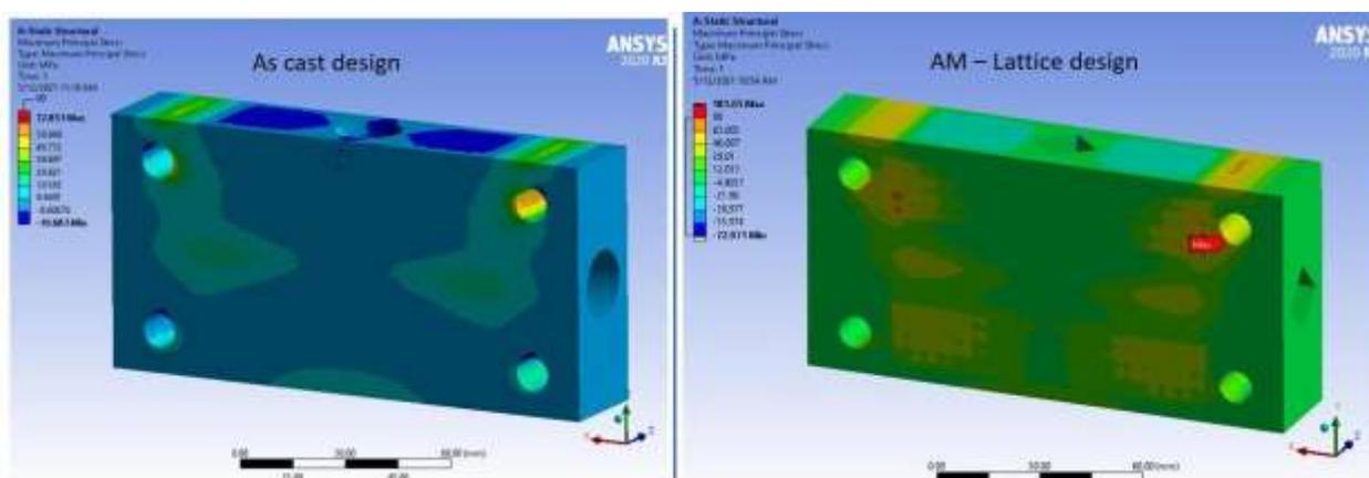
**Fig. Principal stress under pressure load**
