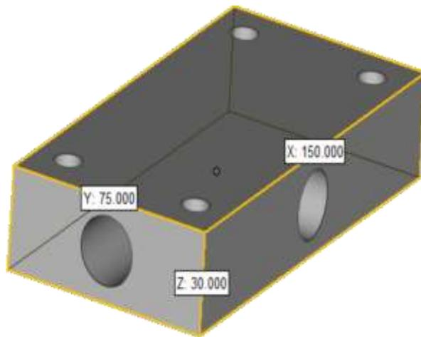
**Fig 3.3 Conventional Design of Hydraulic Manifold**
