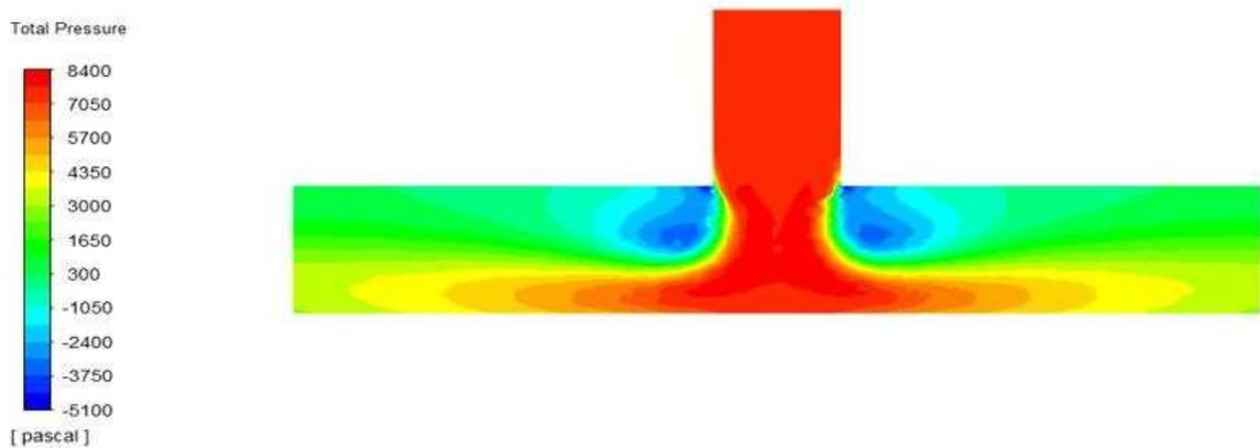
**Fig. Pressure drop in the manifold**
