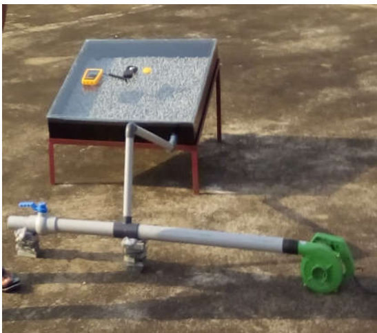
Fig. 2.2 Solar collector with pebbles absorber
