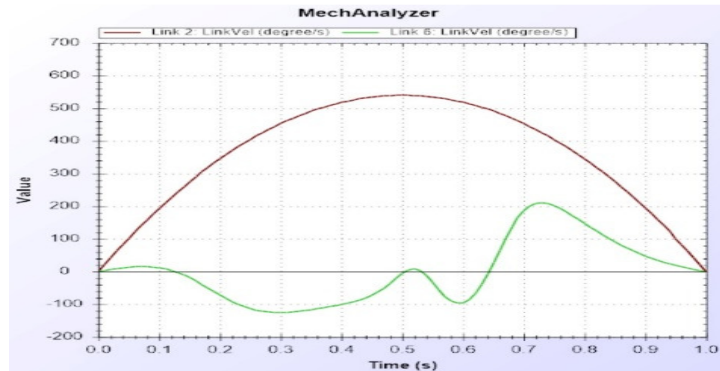
Figure 15. Crank vs End effector angular velocity
