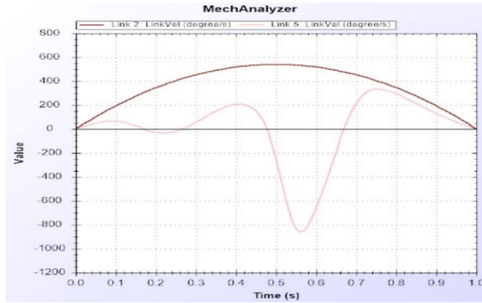
Figure 20. Crank vs L4 angular velocity
