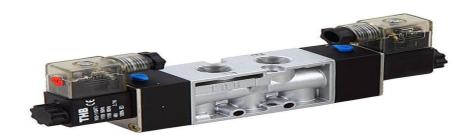
The directional valve is one of the important parts of a pneumatic system. Commonly known as DCV, this valve is used to control the direction of air flow in the pneumatic system. The directional valve does this by changing the position of its internal movable parts. This valve was selected for speedy operation and to reduce the manual effort and also for the modification of the machine into automatic machine by means of using a solenoid valve.
