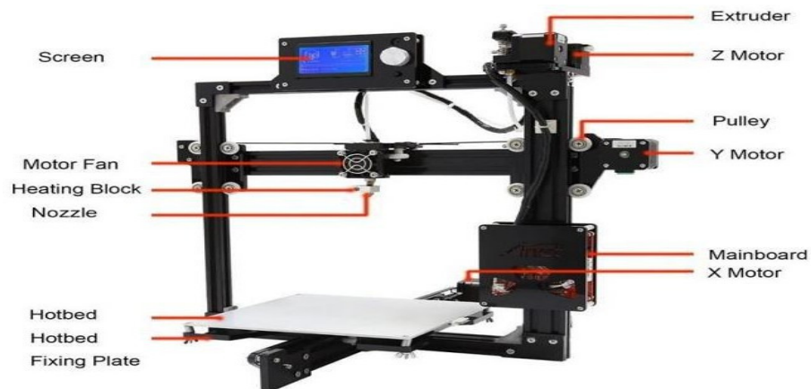
Fig3.2 Parts of 3D Printer
