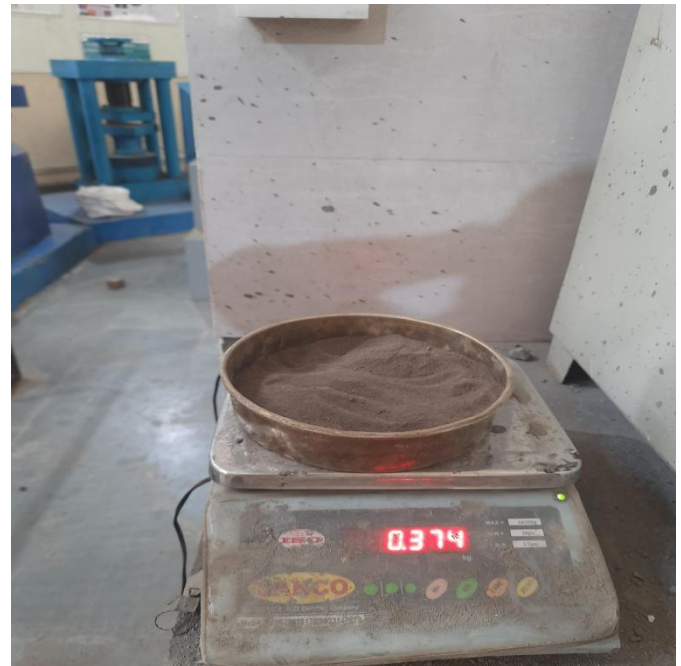
Sewage after Incineration and crushing.
